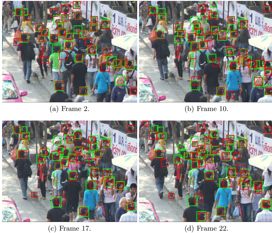
Fig. 3. Sample tracking results on the Mochit test video. Red rectangles indicate estimated head positions, and green rectangles indicate ground truth head positions.
