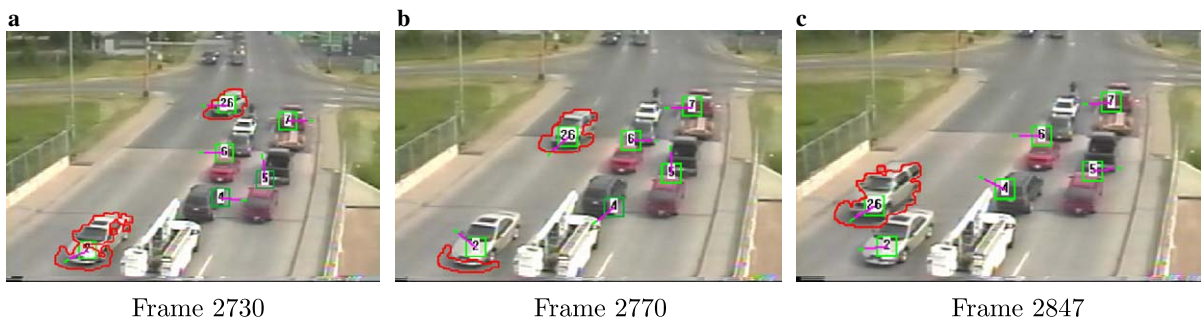
Fig. 8. Scene III: tracking in a crowded scene with stopped vehicles. The contours around the vehicles indicate the blobs detected. For vehicles not having the blob contour, the blob cue was missing.
