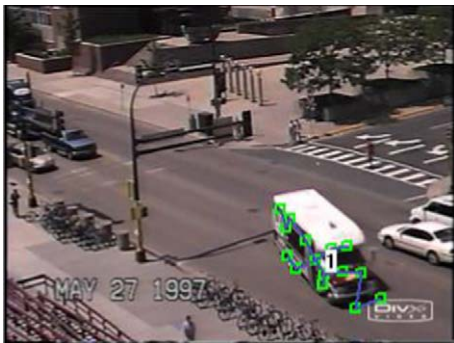
Fig. 4. A geometric template imposed on targets. The template consists of a spanning tree connecting the individual features on the target.
