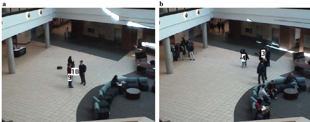
Fig. 11. Tracking pedestrians in an indoor scene. The pedestrians are tracked despite very similar background color and the occluding foreground.
