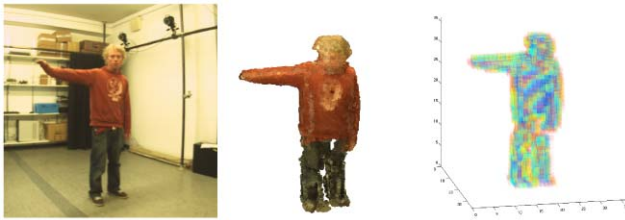
Fig. 3 Example of a reconstructed 3D hull of the user
