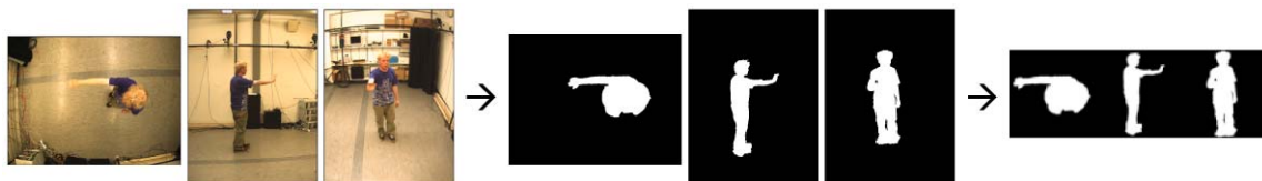
Fig. 2 Example of 3 camera views, foreground-background segmentation, and their concatenation to a single normalized sample
