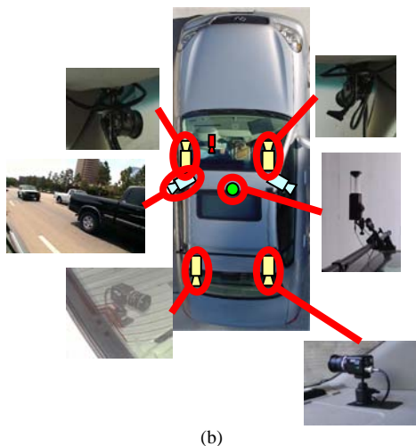
Fig. 2 (a) LISA-P testbed used for occupant and driver posture analysis, and pedestrian detection (b) LISA-Q testbed used for vehicle surround, lane tracking, and driver support system.
