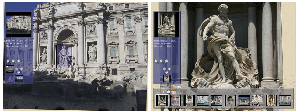
Fig. 5 Object-based navigation. The user drags a rectangle around Neptune in one photo, and the system finds a new, high-resolution photograph
