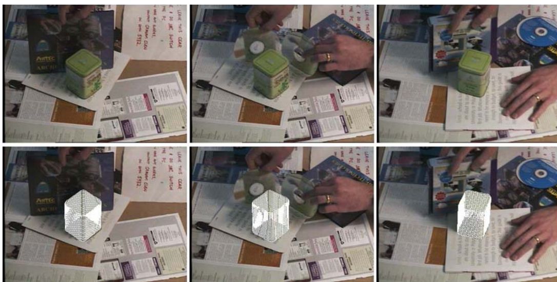
Figure 5. Top row: Input images for frames 51, 189 and 450 of an image sequence containing 560 frames. Bottom row: Pose results. The algorithm is able to deal with a cluttered and changing background.
