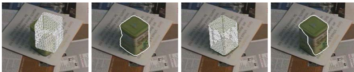
Figure 4. From left to right: (a) Initialization. (b) Segmentation result with object knowledge. (c) Pose result. (d) Segmentation result without object knowledge.
