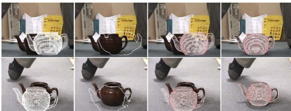
Figure 10. From left to right: (a) Stereo image with a teapot. The initialization is quite far away from the object. (b) Resulting contour when performing only one iteration. The contour is restricted to the initial, bad pose and cannot fully capture the object. (c) Consequently, the pose remains close to the initialization. (d) Pose result after 20 iterations.
