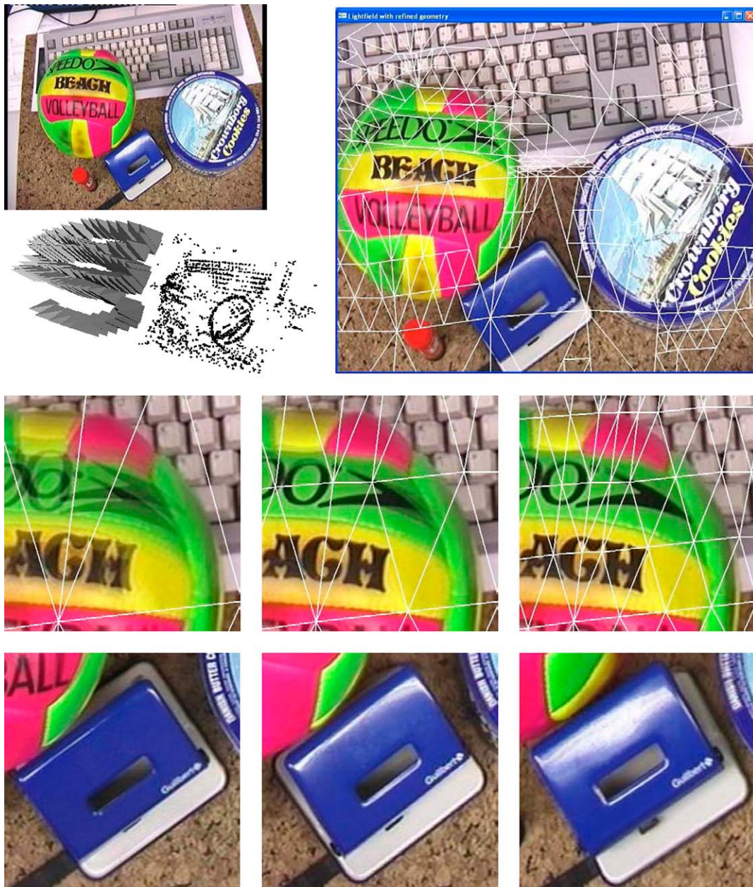
Figure 11. Top: Image of the desk sequence and sparse structure-and-motion result (left) and view rendered using adaptive subdivision (right). Middle: Details of rendered images showing multiple levels of geometric refinement. Bottom: Rendering of a view-dependent effect.
