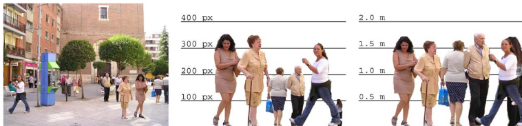
Figure: automatic object height estimation result, (left) picture from LabelMe (center) original pixel size (right) automatically estimated 3D height ( y_i )
