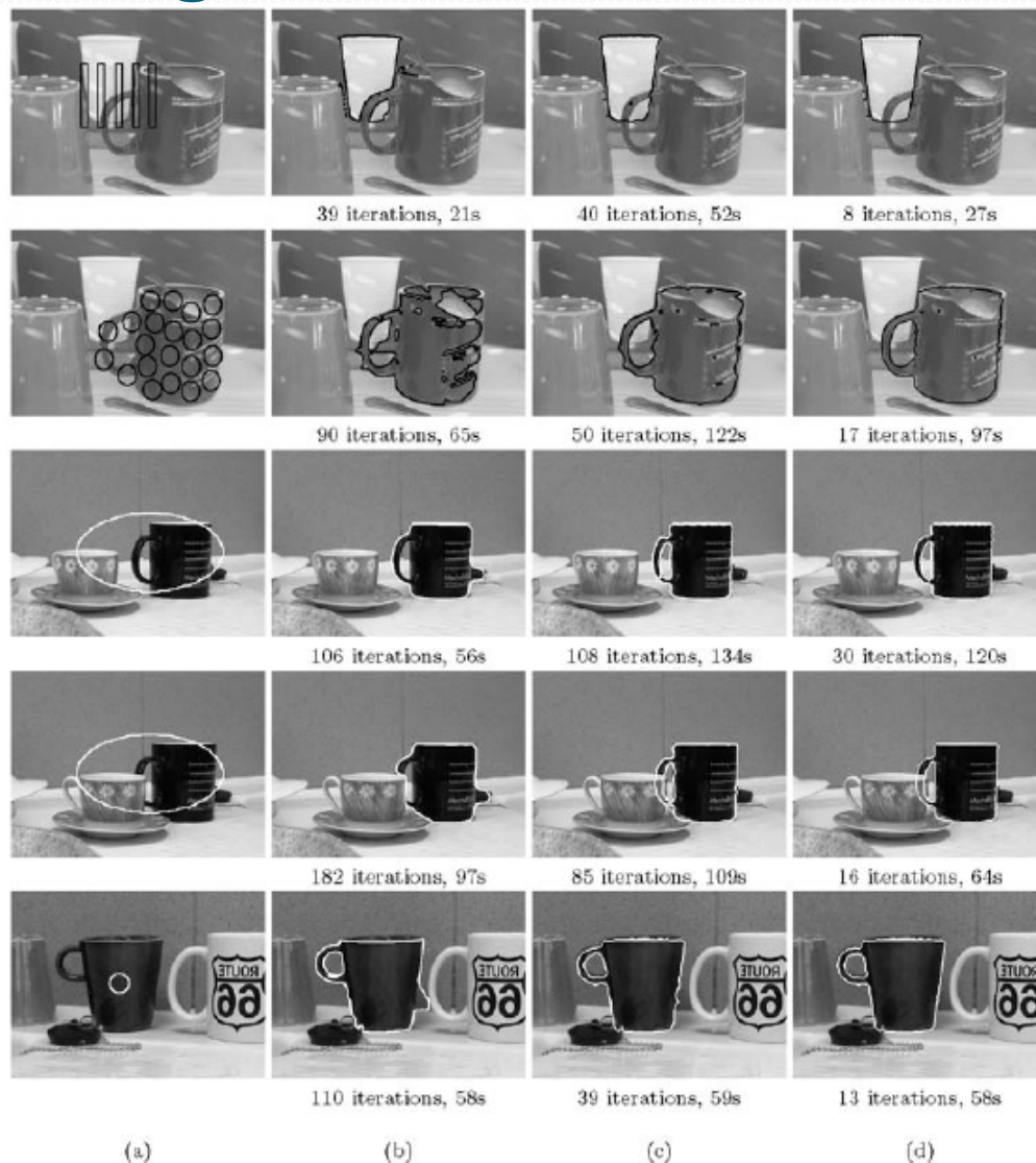
Fig. 8 Segmentation of real images. (a) Initial contours, (b) segmentation results without shape prior (standard curvature component used), segmentation result using the multi-reference prior invariant to scaling and translation: (c) moments up to the 20th-order and (d) to the 40th-order ( \beta = 0.8 ). The number of evolution iterations performed at each stage and the corresponding computation time are given underneath each result
