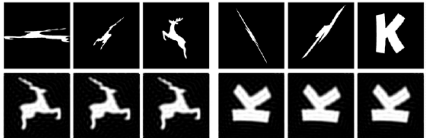
Fig. 2 Reconstruction of shapes from their affine-invariant moments. Upper row : original shapes. Lower row : shape reconstructions using affine invariant moments (these reconstruction correspond to the canonical representations of the original shapes)
