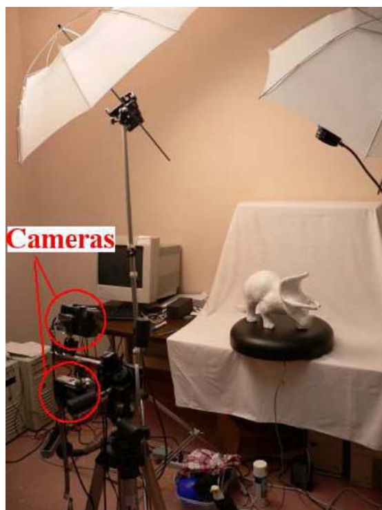
Figure 4. Photograph of our laboratory setup. Each object was placed on a computer-controlled turntable which can be rotated with 1/50 degree resolution and 10^{-5} degree accuracy. Two computer-controlled cameras imaged the object. The cameras were located 10^\circ apart with respect to the object. The resolution of each camera is 3 Mpixels. In addition to a neon tube on the ceiling, two photographic spotlights with diffusers are alternatively used to create 3 lighting conditions.
