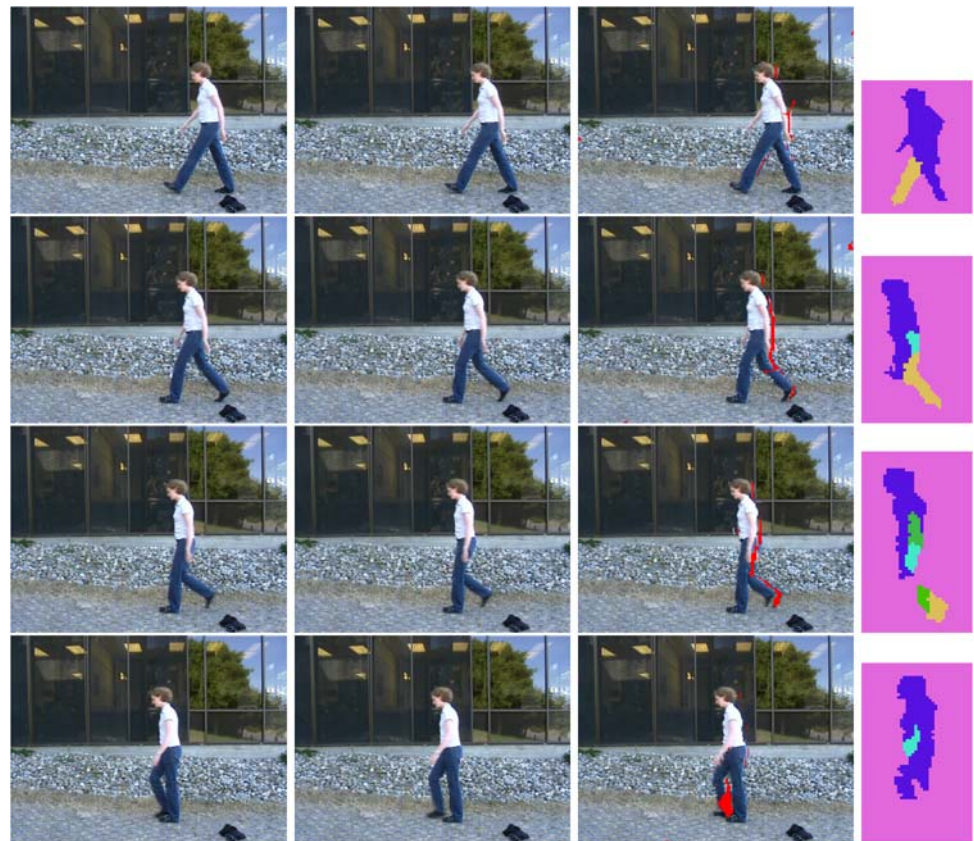
Fig. 6 Results of obtaining the MMSE estimates of the transformations. The first two columns show consecutive frames of a video. The third column shown the reconstruction of the second frame obtained by mapping the patches of the first frame according to the transformations obtained using coarse-to-fine efficient LBP. Points which are occluded from the first frame but are present in the second frame would be missing from the reconstruction. These points are shown in red . Fragments moving rigidly are clustered together to obtain the components shown in the fourth column (Colour figure online)
