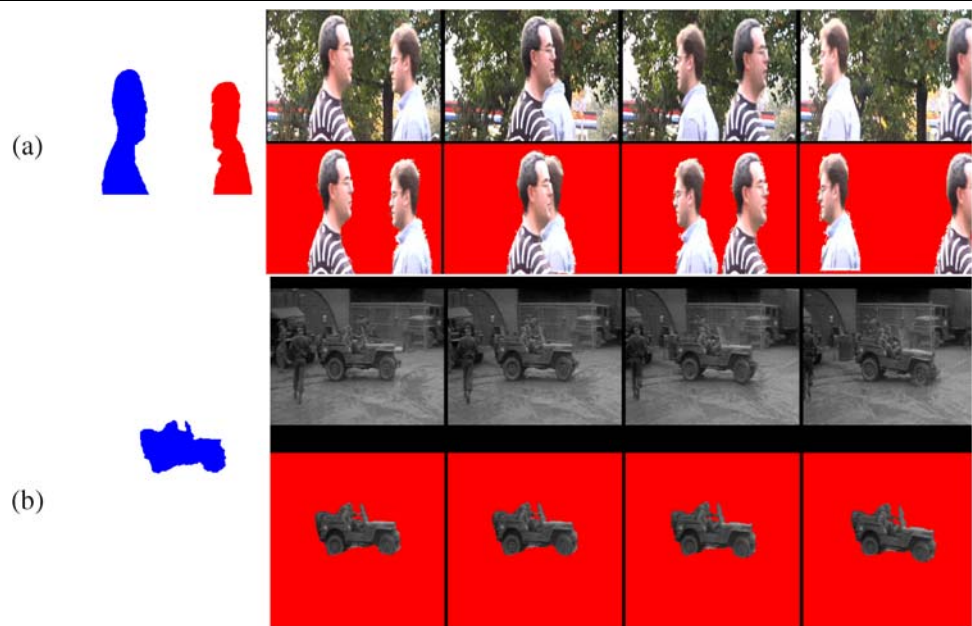
Fig. 14 Motion Segmentation Results I. In each case, the left image shows the various segments obtained in different colors. The top row shows the original video sequence while the segmentation results are shown in the bottom row . a A 40 frame sequence taken from a still camera (courtesy Nebojsa Jojic Jojic and Frey 2001). The scene contains two people undergoing pure translation in front of a static background. The results show that the layering is learnt correctly. b A 10 frame video sequence taken from ‘M.A.S.H.’. The video contains a jeep undergoing translation and slight out of plane rotation against a static background while the camera pans to track the jeep
