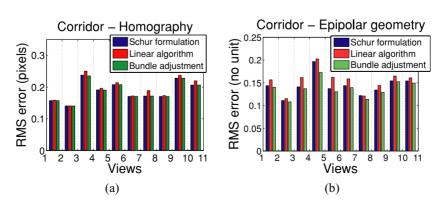
Figure 4. Estimation results of homographies (a) and two-view epipolar geometries (b) for consecutive images in the corridor sequence.
