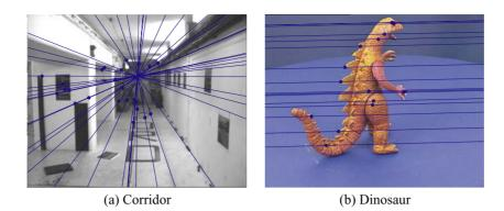
*Figure 3.* First images of the corridor (a) and dinosaur (b) sequences with epipolar lines with respect to the second view. While the first camera is moving forwards (or backwards), the other one is moving sideways.
