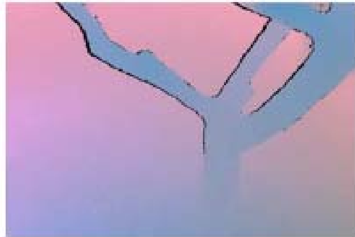
Fig.5 shows flow field generated by optical flow algorithm. Each flow field is generated between a video frame(left) and the subsequent video frame. The flow field is visualized (right) using hue to denote flow direction and saturation to denote flow magnitude. The black regions are labeled by the algorithm as occluded.
