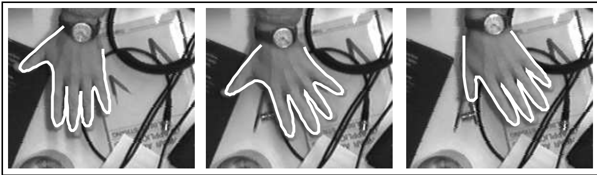
Figure 16: Tracking a flexing hand across a cluttered desk. Representative stills from a 500 field (10 second) sequence show a hand moving over a highly cluttered desk scene. The fingers and thumb flex independently, and the hand translates and rotates. Here the CONDENSATION algorithm uses N = 1500 samples per time-step initially, dropping gradually over 4 fields to N = 500 for the tracking of the remainder of the sequence. The mean configuration of the contour is displayed.
