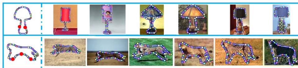
Fig. 11 Refined object descriptions using pairs and triplets of landmarks. In the top row , the user selects two landmarks from the model on either side of the lamp base (highlighted on the left) and asks for the distance between them in test images. Results are displayed in order of this distance increasing from left to right. In the bottom row ,
