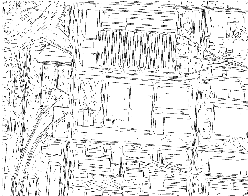
Figure 18. RADIUS model board image J3. The Boldt straight line extraction algorithm produced 2734 lines.
