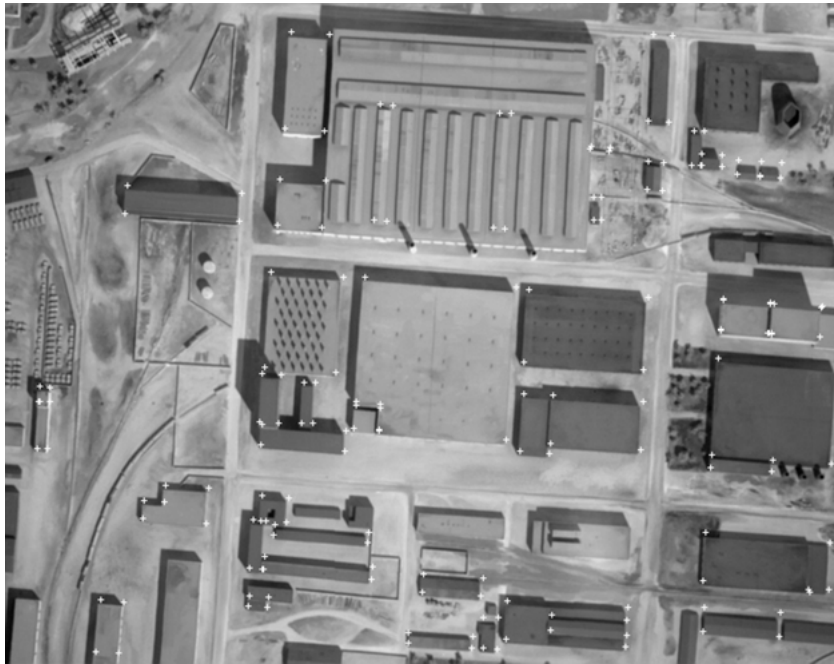
Figure 9. Extracted image points in image J3. The 186 points are a result of generating 2D building polygons via the ASCENDER system.
