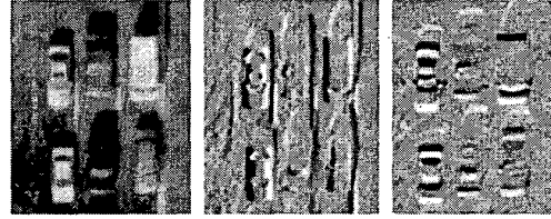
Figure 4: An image patch and its X/Y gradient maps. (in gradient maps, mid gray - 0, white - positive, black - negative) Expected feature values vary with the intensity of the car and shadow. Comparing the bottom three cars, all the features of the white car are clear; the top and right boundaries of the black car are invisible; the left boundary of the gray car is faint; the windshields of the black car and white car exhibit different sign in gradient maps.
